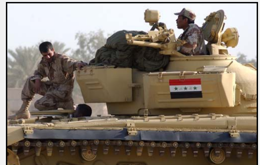
The T-72s can be operated by a three-man crew, travel up to 60 kilometers an hour and fire eight rounds per minute.
